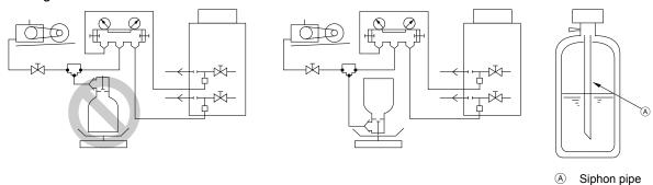
• After evacuation and refrigerant charging, ensure that the service valves are fully open. Do not operate the unit with the service valves closed.
